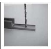
In the basis of the guide drill the holes for the mounting screws at intervals of 10 cm beginning and ending 2 cm from the ends of the guide.
