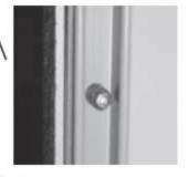
Drill hole ø 3mm depth 11-12 mm, stick the pin.
