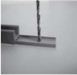
In the basis of the guide drill the holes for the mounting screws at intervals of 10 cm beginning and ending 2 cm from the ends of the guide.
